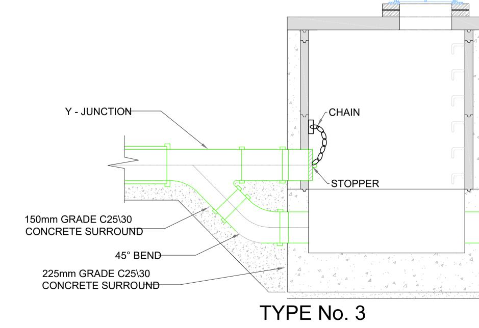
150mm - 450mm DIA. (INCL.) DROP GREATER THAN 600mm AND LESS 500mm - 900mm DIA. (INCL.) DROP GREATER THAN 600mm AND LESS
